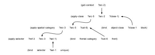
Fig. 2. Example of a network of cognitive operations as needed for interpreting the German sentence "der vordere Block" (the front block). Each cognitive operation has a number of arguments (indicated with a question mark in front of them) which are to be filled by specific values. The arrows indicate that there are data flow relations between the different cognitive operations.
